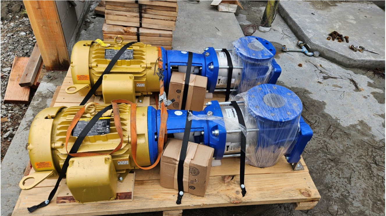
(2) New 25 HP Water Pumps
