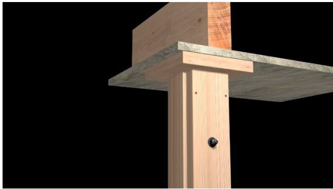
Covered Column Showing Existing Header
